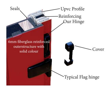
This 3D generated photo demonstrates the advantage of our unique hinge. As is evident from the above picture, this hinge is not attached to the outside of the door, and therefore enhances the appearance of the door, unlike a more conventional flag hinge - as seen on the left. Double seal and rebate.
